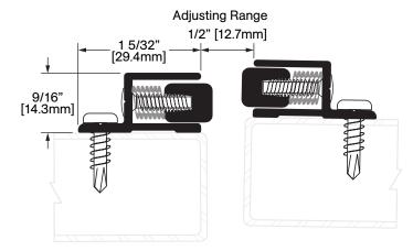
**Operation:** Adjustable Astragal Features: Clear Anodized Extruded Aluminum Application: Ideal for Residential, Commercial & Industrial Maximum Length: 120 in [3048 mm]
