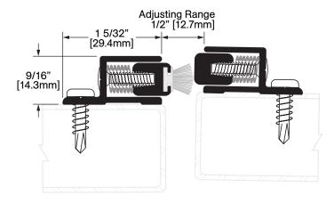
**Operation:** Adjustable Astragal Features: Clear Anodized Extruded Aluminum with Pile on one side only Application: Ideal for Residential, Commercial & Industrial Maximum Length: 120 in [3048 mm]
