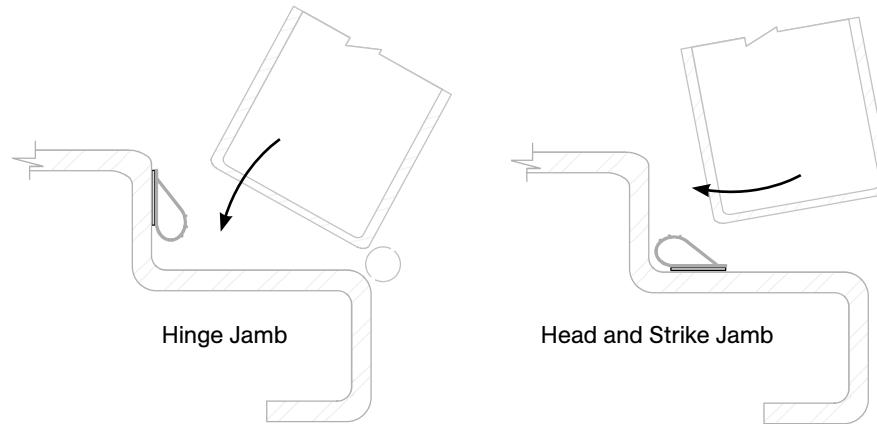
**Operation:** Self-Adhesive Weatherstrip Gasketing for Fire Doors**Features:** Silicone Self-Adhesive Gasket
