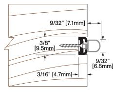
**Operation:** Astragal Features: Mill Finish Extruded Aluminum with Neoprene Insert Application: Ideal for Residential, Commercial & Industrial Maximum Length: 144 in [3658 mm]
