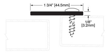
**Operation:** Astragal Features: Primed C.R. Steel with Conditioned Edges Application: Ideal for Residential, Commercial & Industrial Maximum Length: 144 in [3658 mm]
