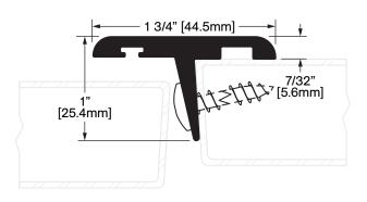
**Operation:** Astragal Features: Clear Anodized Extruded Aluminum Application: Ideal for Residential, Commercial & Industrial Maximum Length: 120 in [3048 mm]
