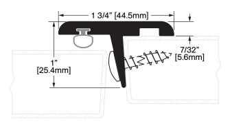
**Operation:** Astragal Features: Clear Anodized Extruded Aluminum with Neoprene Application: Ideal for Residential, Commercial & Industrial Maximum Length: 120 in [3048 mm]
