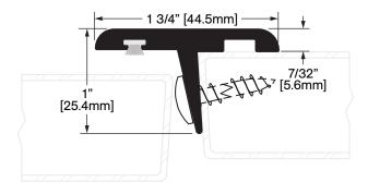
**Operation:** Astragal Features: Clear Anodized Extruded Aluminum with Pile Application: Ideal for Residential, Commercial & Industrial Maximum Length: 120 in [3048 mm]
