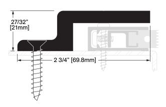
**Operation:** Door Closer Mounting Bracket Features: Clear Anodized Extruded Aluminum
